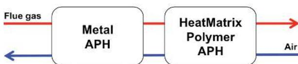
**Figure 4.** Metal and polymer air preheater in series.
