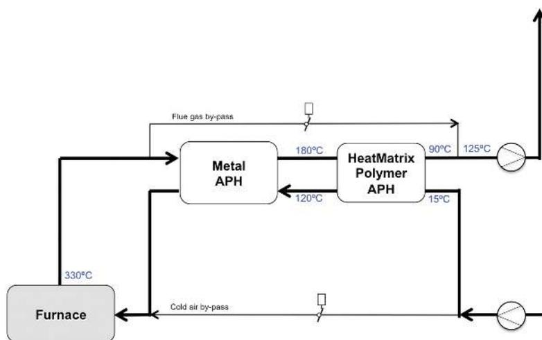
**Figure 5.** Process diagram of a metal and polymer air preheater assembly.
