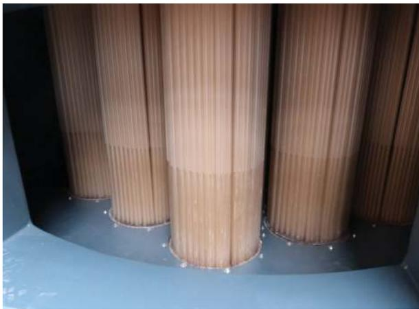
**Figure 2.** Polymer tube bundles.
